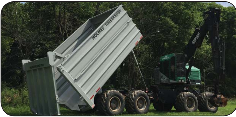
TimberPro 840 fitted with a special dump body for removing jobsite debris and biomass.
