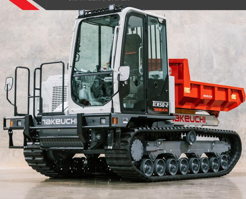
Operating Weight • 14,440 lb **Dump Body Capacity** 2.7 cu yd Max Loading Weight - 8,157 lb
